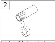
2. Apply pipe Teflon tape on the pipe nipple threads.
