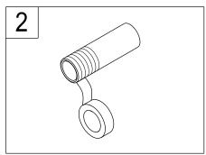
2. Apply pipe Teflon tape on the pipe nipple threads.
