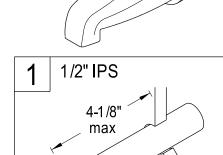
The stub-out pipe for spout installation must be at the length illustrated measured from the finished wall surface.
