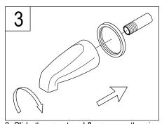
3. Slide the spout and flange over the pipe. With the spout tight to the wall, tighten the set screw to the pipe.
