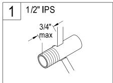
The stub-out pipe for spout installation must be at the length illustrated measured from the finished wall surface.
