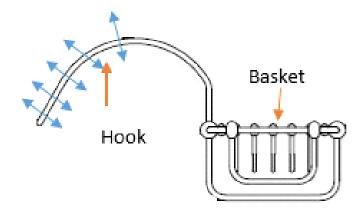
While holding the basket with one hand, grab the hanger hook and bend it slightly, place it on the tub, if the basket is still sagging, re-adjust the hook as necessary.
