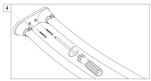
4. Place the shower rod on the mounting location and insert screws through first mounting post into anchors. Tighten screws with screwdriver.
