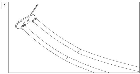
1. Locate where you would like to install the curved shower rod. Place a base onto the wall and trace around it with a pencil.
