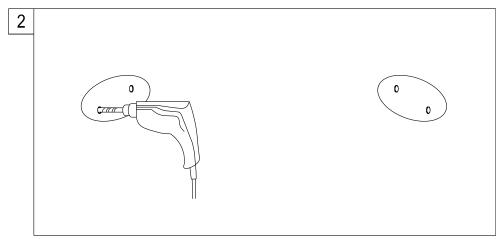
2. Place the mounting plate in the center of the pencil outline you just made and mark the location of the mounting screws. Drill holes at the marked locations.
