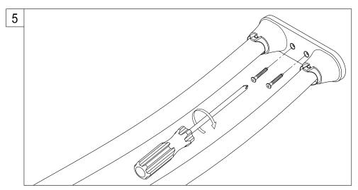
5. Expand the shower rod and install on opposite end. Repeat steps 1 through 4 with the other side.
