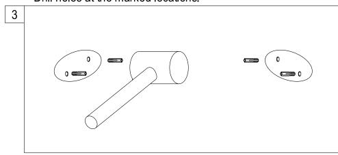
3. Insert anchors into the holes with a hammer until flush with the wall.
